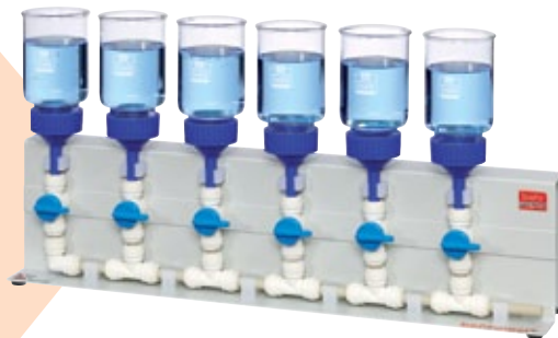
Filter equipment for hydrolysis p. 18
