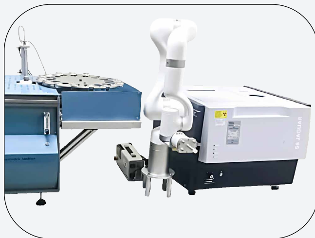
Automated fusion system with XRF spectrometer and collaborative robot arm
