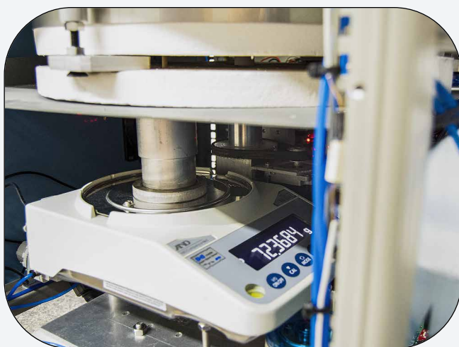
Balance pedestal located inside furnace base
